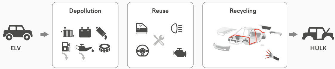
FIGURE 9. Regular compliant and profitable dismantling process at INDRA Re-source
