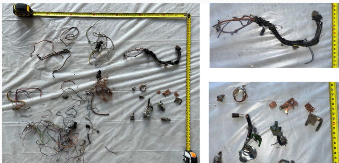
FIGURE 20. Detail of the copper fraction of sample E3 (left), close-ups of the largest cables, connector elements and small inductors (right).
